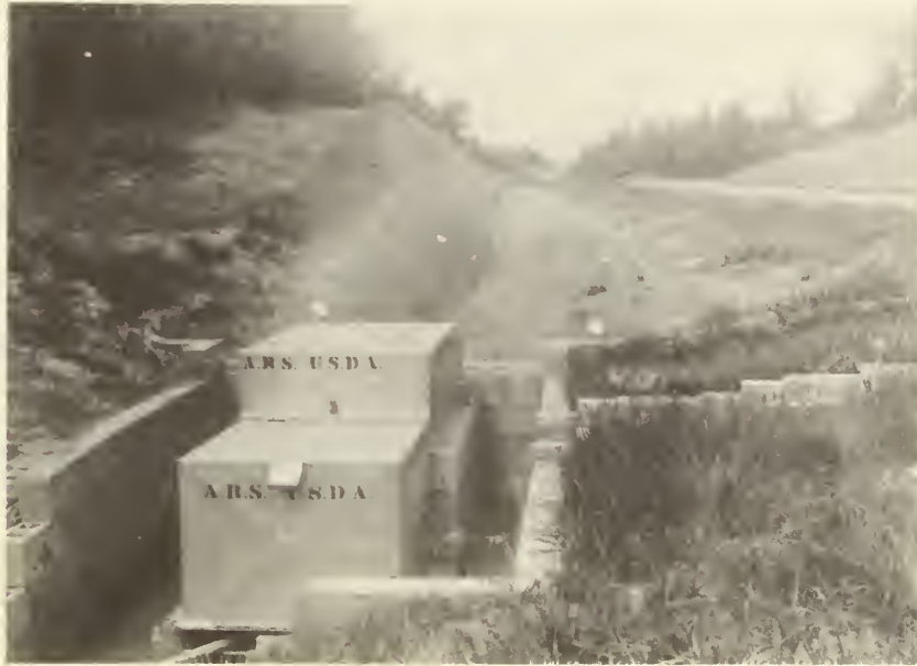
Figure 2.--View of a soil and water measuring device installed at the lower end of a plot ditch for measurement of losses occurring from highway cut slopes. The bare road cut and ditch are shown in the background where the white papers appear.
